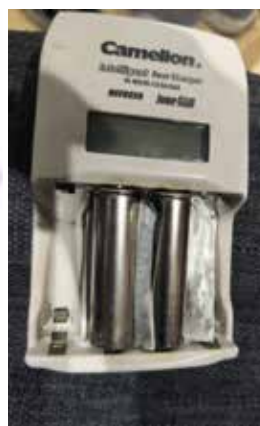
The overheated batteries in the charger, and David's burned fingers
