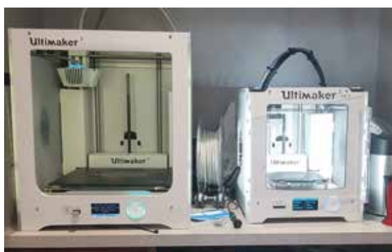
From left, Fusion screenshot showing sketches and 3D object; Ultimaker 3 and Ultimaker2Go 3D printers, with reel of filament in between; Cura screenshot showing model in virtual printer
