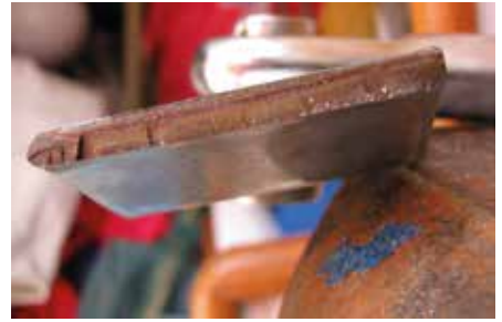
Left, a mast tang and right, a mast tang showing "beach marks" which are characteristic of fatigue failure
