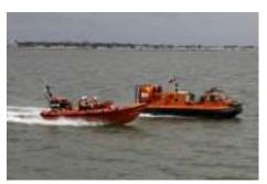
of four operated by the RNLI in the UK. It is used in areas of tidal mudflats where the surface is too soft to support land vehicles and the water too shallow for boats.
